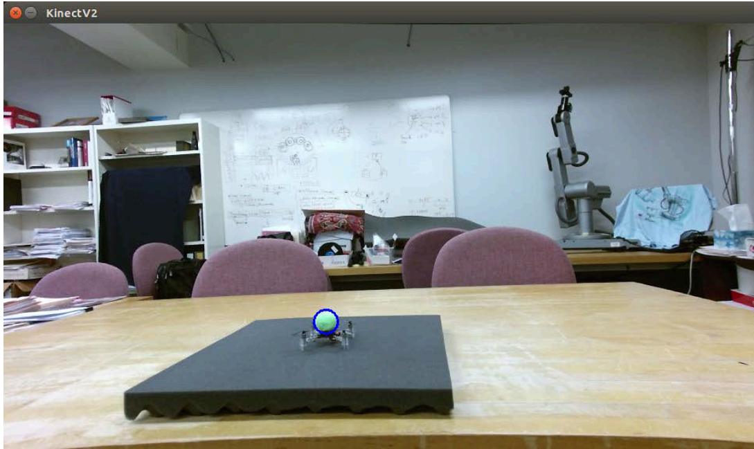
Figure 2: Kinect recognizes the marker attached to the Crazyflie (C. Fairchild, T. Harman, 2016)
